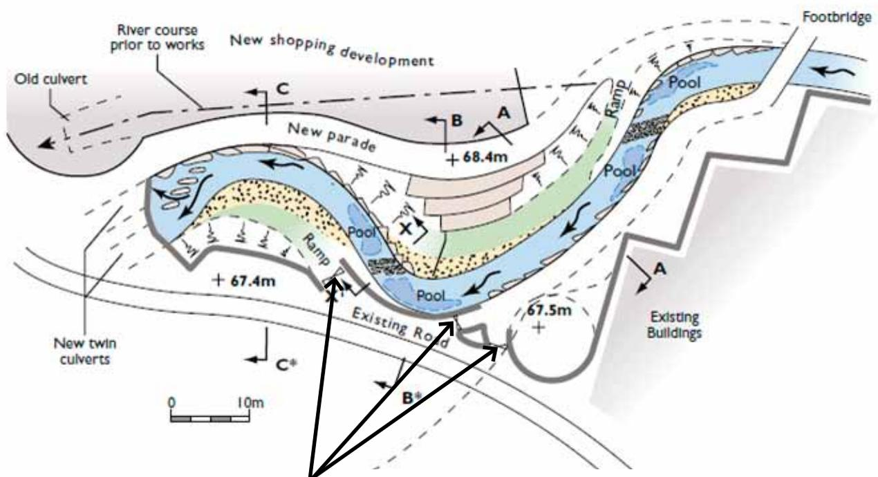
Flood gates that can be closed off to prevent the town from flooding during high water and prevents public access during these events
