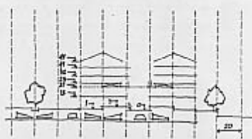
Figure 4. The cross-sections of Figure 2 are minimal cross-sections. They give a backyard space — including the fire lane — from building to building of 80' nominally with four large modules. Other larger dimensions could have been chosen. Each dimension includes from four to seven large modules and gives its own possible arrangement of cars and lanes in the garage space.
