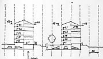
Figure 5. Gives rules on vertical dimensions. On the left-hand we have again the building along the raised residential street. If the ground floor is for commercial use it should be at sidewalk level. The right-hand sections give the same building but this time with a raised floor along the sidewalk. This should be adopted if a dwelling is to be on the first floor.
